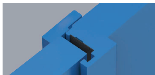
Horizontal cross section of the central rebate
